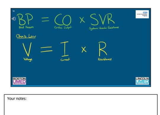
This is Ohm's Law, which in electronics governs the relationship between Current, Resistance, and Voltage.
